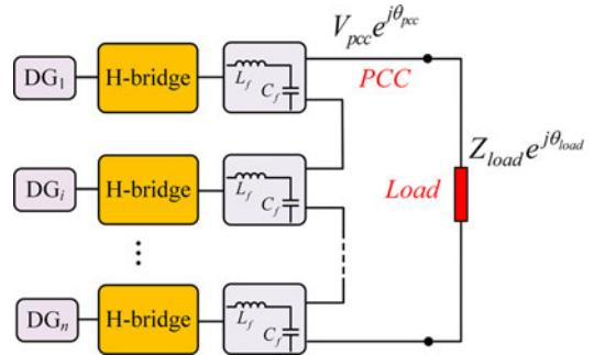
Fig. 1. Structure of islanded cascaded-type microgrid.
