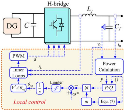
Fig. 2. The local control diagram of the  $i$ -th DG.
